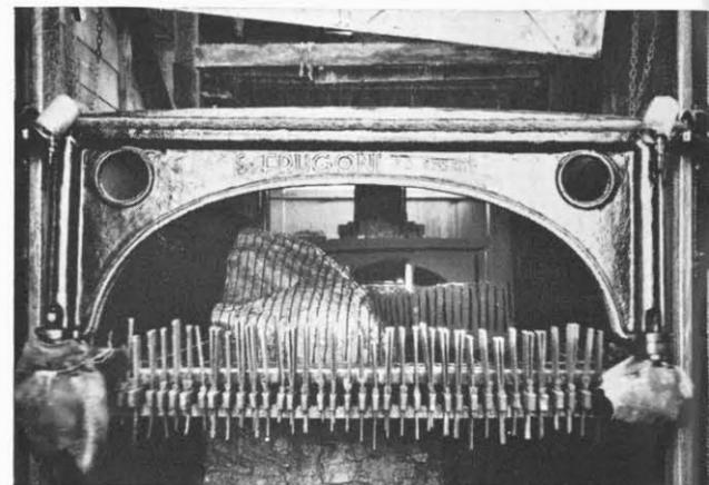
Steel blades of slicing equipment gradually cut through marble so that the boulder is reduced to thin slabs.
