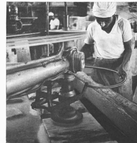
High gloss of finished marble is obtained by hand-guiding a polishing wheel over slab.
