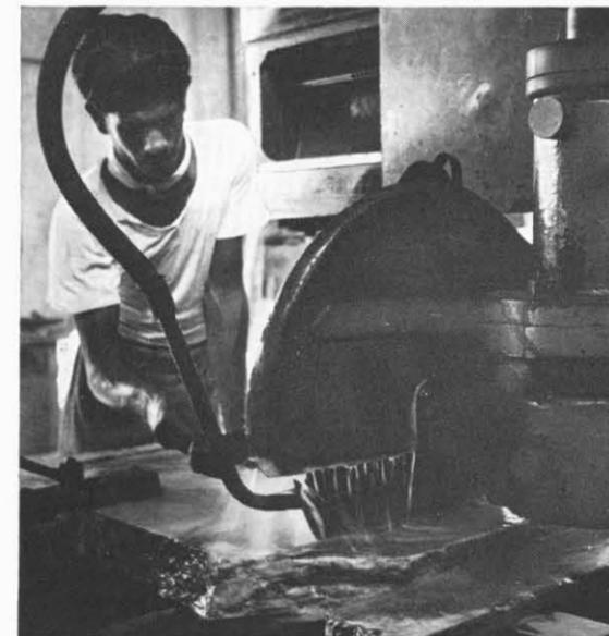
Saudi Arabian marble is extremely hard, but slabs are cut into smaller sizes by tough carborundum-edged wheels.
