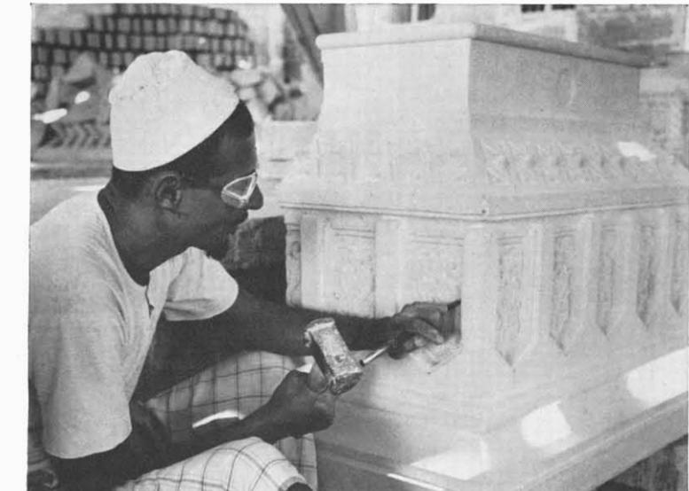
Decorative base of cast marble undergoes refining touches after removal from mold. At left, marble panels in storeyard await further cutting and polishing.
